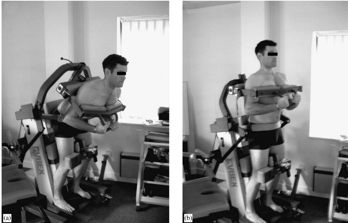
Fig. 2 The Cybex Norm Dynamometer: (a) concentric extension, (b) concentric flexion.
